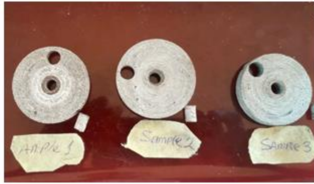
Figure 3: Samples of Epoxy Composites Reinforced with Hybrid Materials: Calabash and Rice Husk Ash
