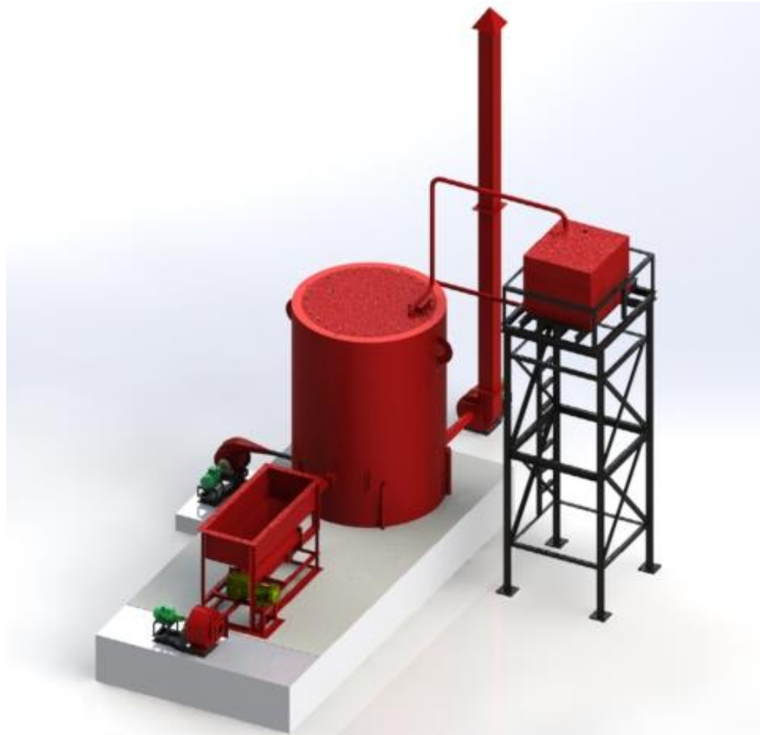
Fig 1: 3D CAD Model of the Steam Boiler
