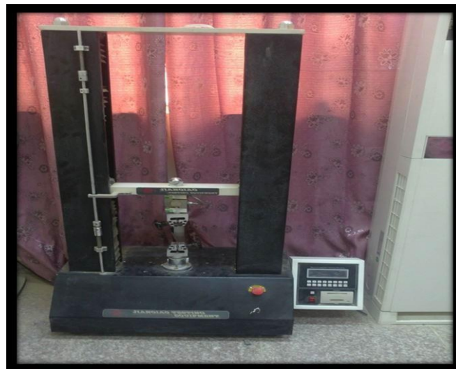
Figure 4: Tension testing device
