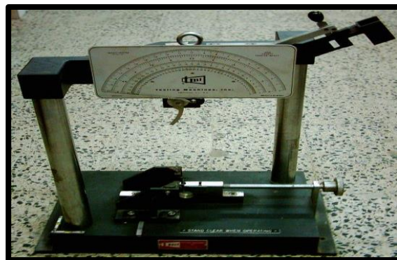
Figure 2: The shock resistance testing device.
