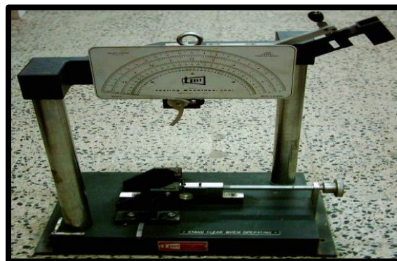
Figure 2: The shock resistance testing device.
