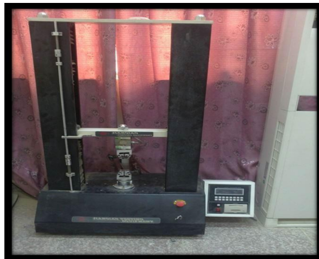
Figure 4: Tension testing device
