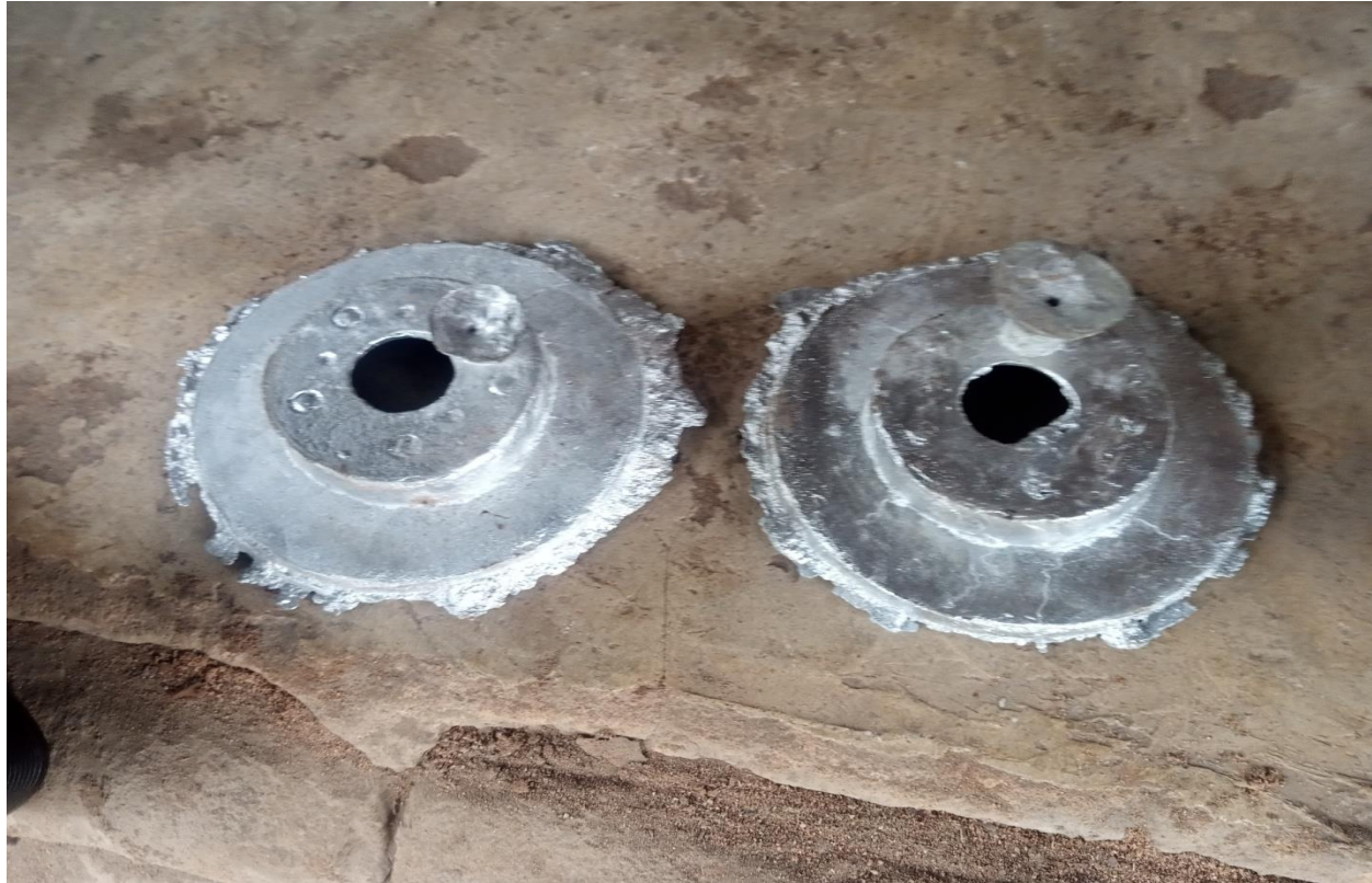
Figure 1: the produced brake disc
