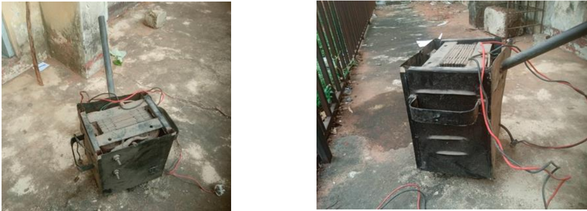
Figure 1: pictorial view of the locally made manually operated shielded metal arc welding (SMAW) system
